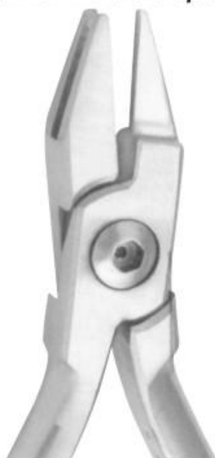
KTS50709 Aderer Clamp three jaw wire bending plier for contouring and bending wire up to .30"/.76mm.
